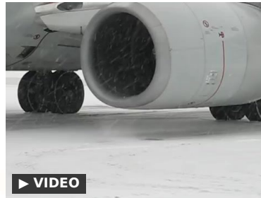
American Airlines ICE_FOD_Vortex (117.9 s). An American Airlines 737 taxiing in falling snow, with a marshaller; close-ups show snow being drawn into the engine inlet. The frames do not show damage or a compressor stall. Still: frame at 90 s, as shared with WheelTug. No watermark visible.
